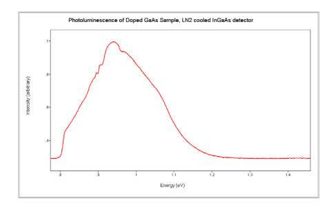
The excitation light is chopped, so that a lock-in amplifier can be used in conjunction with an InGaAs detector for data acquisition. After the initial system alignment is fixed, the experiment itself is controlled by computer using SpectraMax for Windows spectroscopy software.
