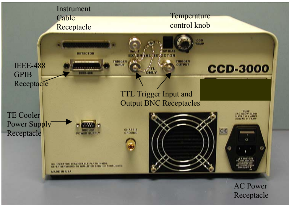
Figure 7b. Rear view of CCD3000V controller, with labeled parts.
