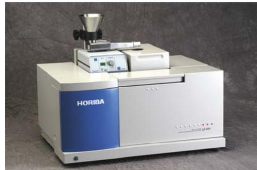
*Horiba LA-930 Particle Size Analyzer with PowderJet Dry Feeder*
