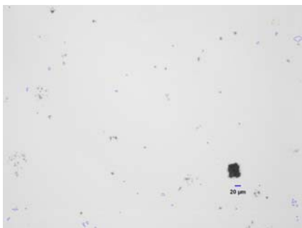
Figure 8: Large Particle from MDI
