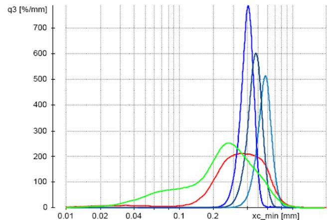
Figure 3: Green: Used sand containing fines and combustion residues. The sand is recycled, cleaned and mixed with new sand (blue) and is then used for new molds (red).
