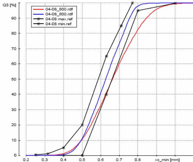
Figure 2: Measurement of filter sand 0.4 – 0.8 mm. Red: CAMSIZER without fitting, Blue: CAMSIZER with elementary fitting. Black Curves: upper and lower product specifications.
