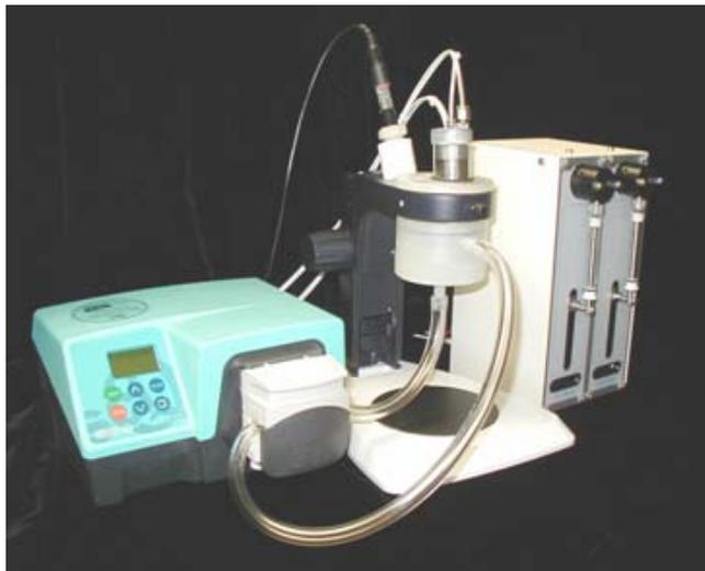
Figure 2: Setup 2 is suitable for all probes except the acoustic sensor used for particle size analysis. The peristaltic pump performs the mixing. The sensor holder is designed so that the sample stream hits the face of the electroacoustic sensor in order to keep it clean. Sonication is possible in this configuration and the sample volume is 150 mL. The probes are easily accessed, but the disadvantage is that particle size analysis is not possible.
