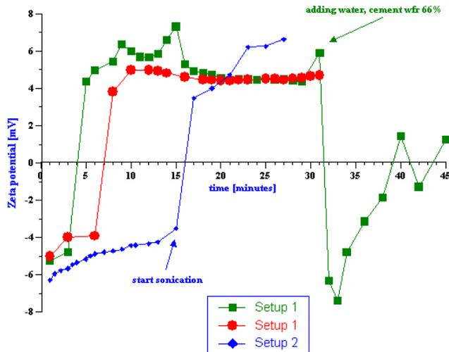
Figure 5: Green and red: zeta potential vs. time using Setup 1 for cement A. Blue: the effect of sonication for cement A using Setup 2.
