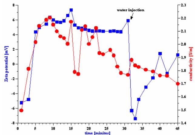
Figure 7: Blue curve: zeta potential vs. time dilution study. Red curve: conductivity vs. time for cement A using Setup 1.
