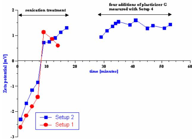
Figure 6: Zeta potential vs. time for cement B using Setup 1 and Setup 2.
