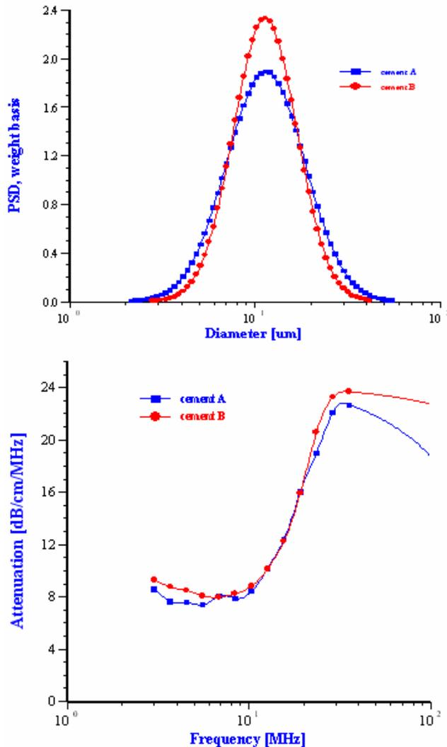
Figure 9: Above: the particle size distributions of cement A and cement B. Below: the attenuation spectra for cement A and cement B.
