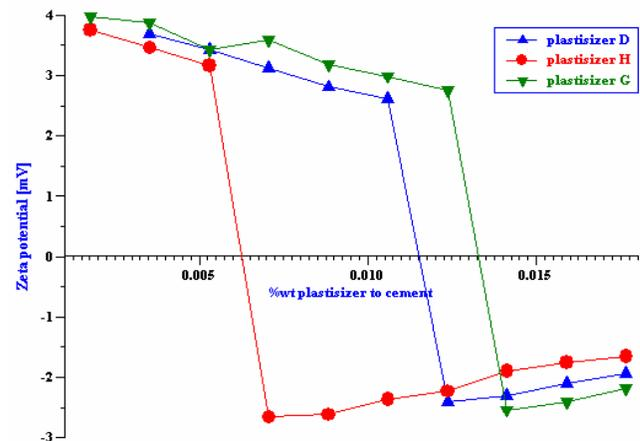
Figure 8: Zeta potential of three super-plasticizers at different concentrations.
