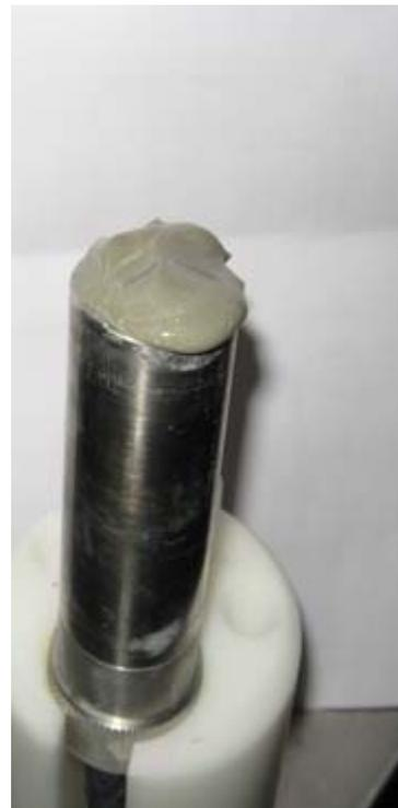
Figure 4: Setup 4 is the simplest configuration for measuring zeta potential. This setup was used at the end for measuring the effect of super-plasticizer on the cement zeta potential. There is no difference between data obtained from this configuration and that of Setup 3. The sample is prepared in a separate vessel just the same. A small amount of prepared sample is placed on the face of the electroacoustic sensor to perform the measurements.
