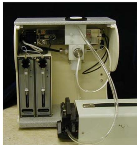
*Figure 1: Setup 1 is based on the standard DT-1201 chassis, making all sensors available. The sonication probe goes on the top of the sample chamber. Mixing is performed with an external peristaltic pump. Two burettes open the possibility of automatic titrations. The sample volume is the largest for this setup, 200 mL. It has the disadvantage of requiring more involved cleaning. Both the zeta potential and conductivity probes could become contaminated if used without care.*
