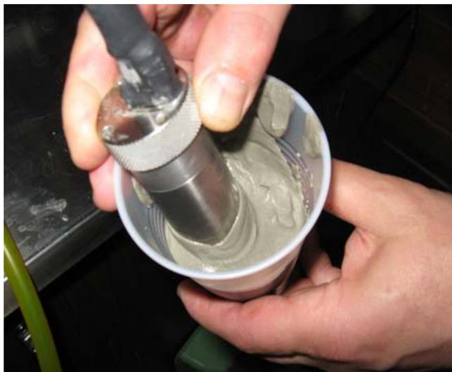
Figure 3: Setup 3 can be used with a sample that has already been prepared (mixed and sonicated) on the side in another vessel. It is suitable for measuring zeta potential only and cleaning is very simple.
