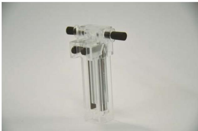
*Figure 2: A carbon coated electrode zeta potential cell, usable after several hundred measurements*
