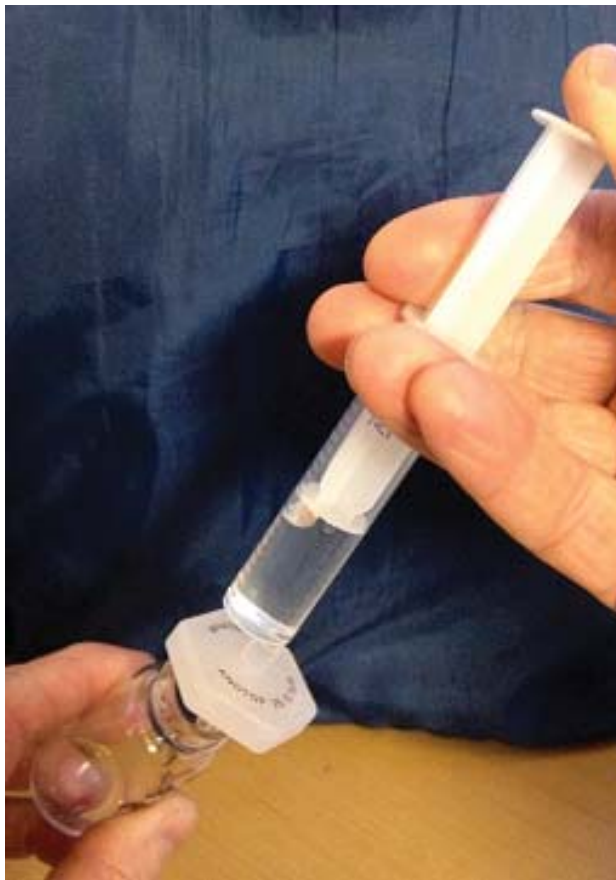
Figure 2: Filtering 10 mm NaCl before adding PSL standard
