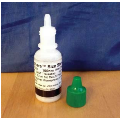
Figure 3: PSL bottle (Note - tip should be pristine)
