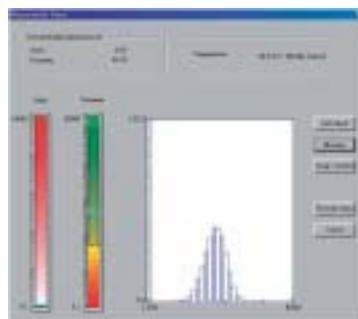
Real-Time Window Display-Particle size distribution information is available immediately after loading the sample cell!
