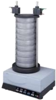
Master sieve stack (that wears with use)
