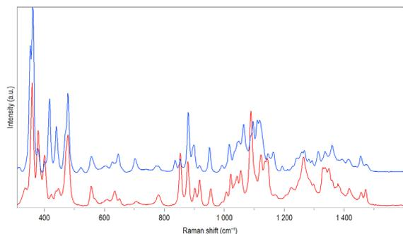
Fig. 2: Raman spectra of *anhydrous lactose* and *lactose monohydrate*.
