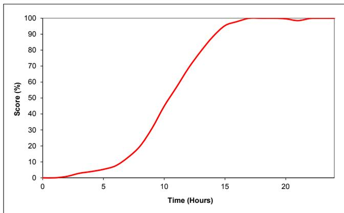
Fig. 7: Scores (%) of the monohydrated form, obtained with the CLS fitting of the averaged spectra of each mapped area.
