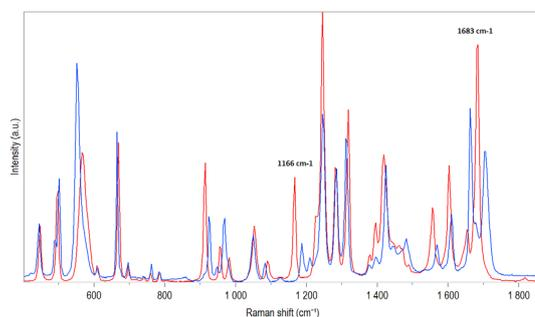
Fig. 4: Raman spectra of the *anhydrous II* and the *monohydrated forms of the theophylline*.
