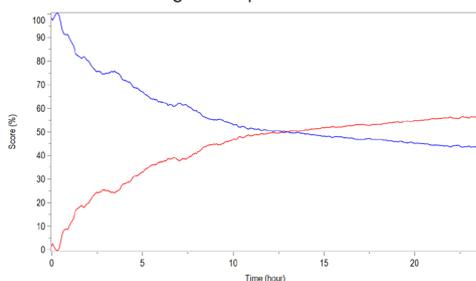
Fig. 3: Scores (%) of *anhydrous lactose* and *lactose monohydrate* obtained from CLS fitting, during a 24h exposure of anhydrous lactose to a relative humidity of 95%.
