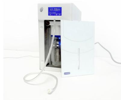
Fig. 1: The Linkam RH95 Humidity Controller.
