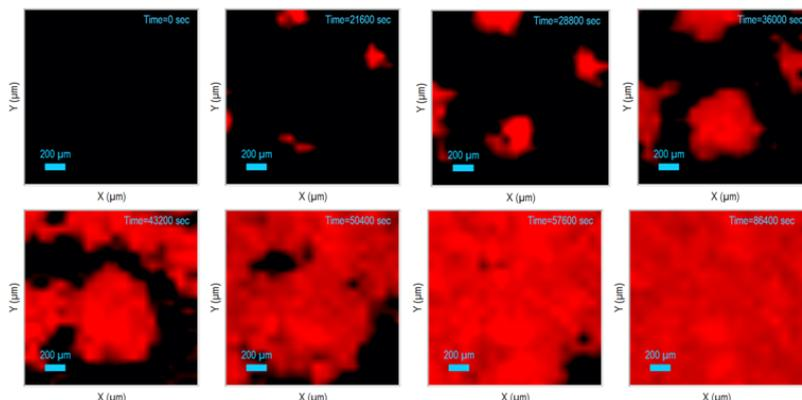
Fig. 6: Raman images of the monohydrated form of the theophylline after different exposure times to 95% RH – 0h, 6h, 8h, 10h, 12h, 14h, 16h and 24h.
