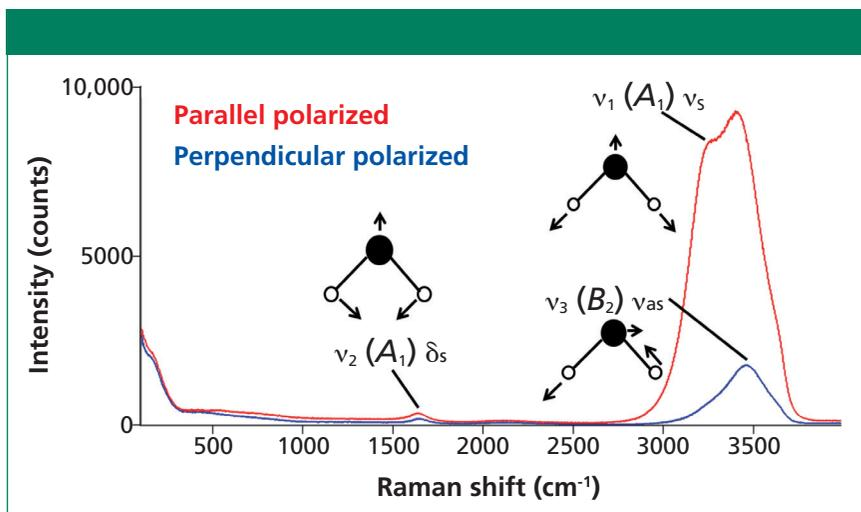
Figure 1: Polarized Raman spectra of H<sub>2</sub>O.
