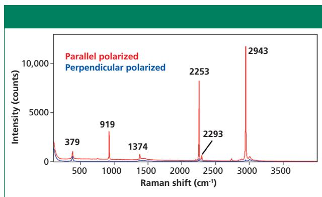
Figure 5: Polarized Raman spectra of acetonitrile.
