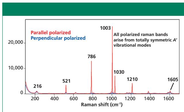
Figure 4: Polarized Raman spectra of toluene.
