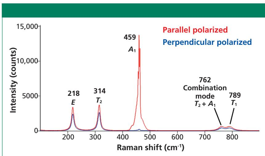
Figure 2: Polarized Raman spectra of CCl<sub>4</sub>.
