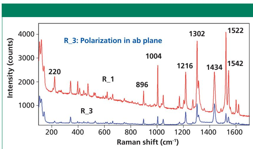
**Figure 8:** Raman spectra of different grains of rubrene.
