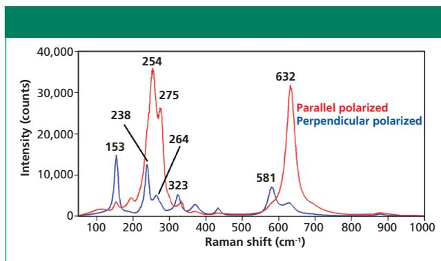
**Figure 6:** Polarized Raman spectra of the *X*-face of single crystal  $\text{LiNbO}_3$  with the incident laser polarized along the *Z*-axis.
