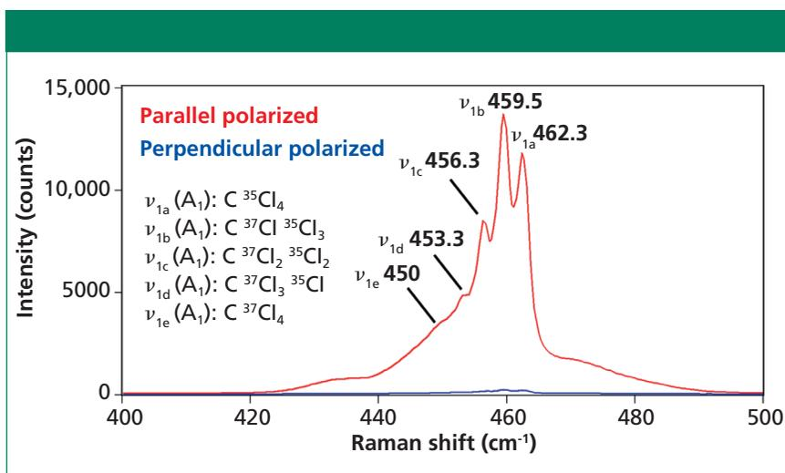
Figure 3: A<sub>1</sub> Symmetric stretching band of CCl<sub>4</sub>. The band is split in accordance with the isotopic abundance of Cl.
