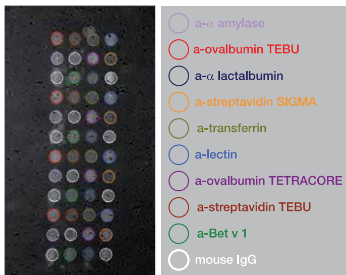
Figure 1: Image of the printed SPRi-Biochip™ and spotting matrix
