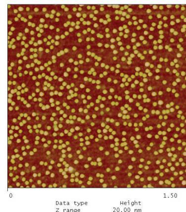
Figure 1: AFM picture of composite layer of Gold nanoparticles into PVA matrix
