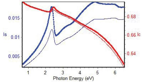
Fig 9b.: Ellipsometric simulations of 15nm Au nanoparticles deposited on SiO<sub>2</sub> with interaction layer activation (dots) and without interaction layer activation (solid line). Surface coverage was 100 particles μm<sup>-2</sup> and density 1%.
