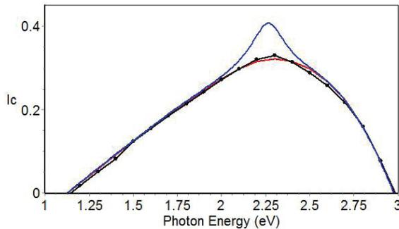
Figure 2: Modeling sample illustrated on Fig1. Experimental data in black dots, standard EMT modeling in blue, improved modeling with electronic confinement in red
