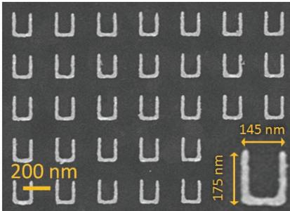
Figure 11: Picture of the array of gold split ring resonators
