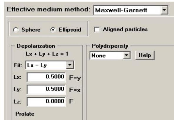
Figure 4: DeltaPsi2 user interface for modeling non spherical shapes of nanoparticles
