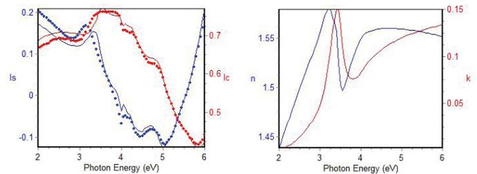
Fig 5a.: Ag Nanowire data and fit results - Fig 5b.: Optical index of the composite film
