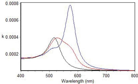
Figure 7: Extinction coefficient for Gold nanoparticle solutions. Spheres (black), Nanorods (blue), Mixture of spheres and nanorods (red)
