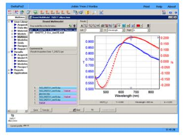
The New Amorphous dispersion formula was used to model the refractive index for TiO<sub>2</sub>.
