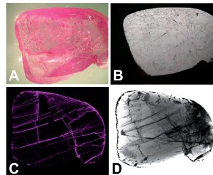
Figure 2: Analysis of ruby (A) optical image by reflection, (B) optical image by transmission, (C) lead XRF image, (D) x-ray transmission image
