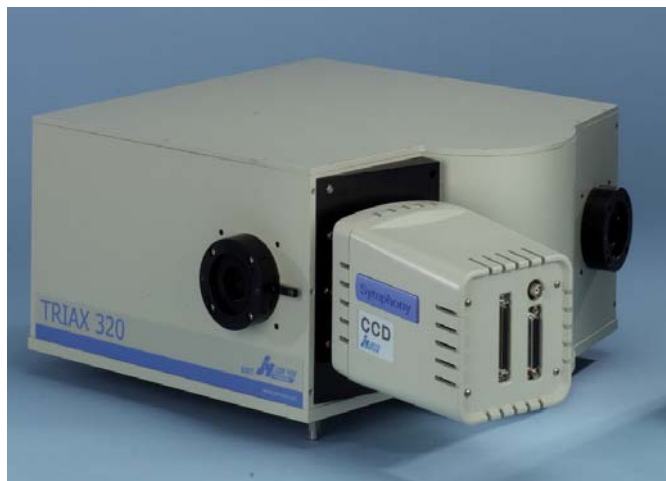
Figure 3. View of Symphony STE Detector Mounted to a Triax 320
