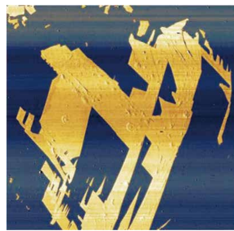
AFM Capacitance image of the same graphene flake
