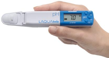
Calibrate and measure at the touch of a button—the smiley face will tell you when the result can be read.
