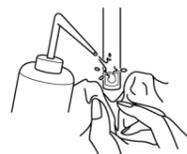
2. Clean the inside of the protective cap with pure water (or deionized water), then add enough pure water (or deionized water) to soak the sponge.
