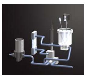
pressure nozzle to disperse agglomerates before delivering the sample stream directly to the measurement cell. This eliminates the sample buildup and contamination found in systems that use a tube feed from the disperser to the measurement cell.
