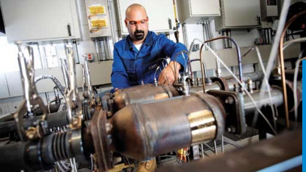
A BASF Catalysts technician sets up a catalyst long-term stress test in the laboratory. Future emissions regulations are expected to require greater catalyst durability.
