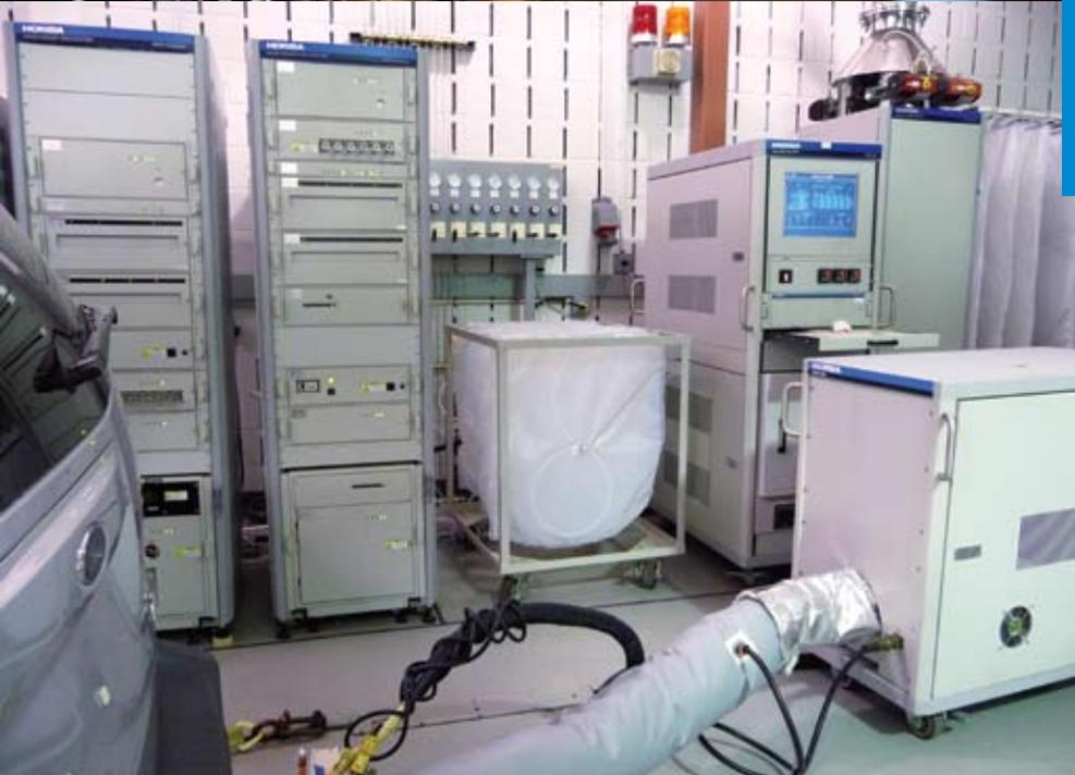
Exhaust test cell showing a Horiba BMD-1000 (at right), the collection bags (center), and the MEXA-7000 (left). In the foreground is the heated sampling pipe coming from the vehicle and entering the EXFM exhaust flow meter. Its measurement determines correct dilution.
