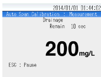
Fig. 26 Display of automatic span calibration result
