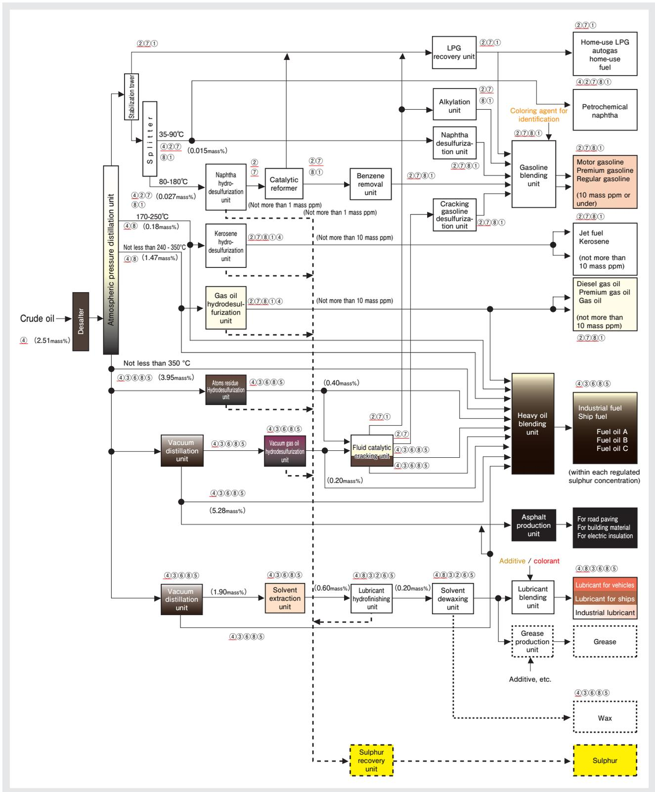
Figure 1 Example of oil refining process
