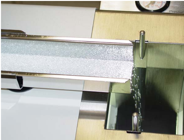
Measurement of glass beads on the Camsizer
