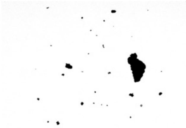
Figure 2: Image collected by the CAMSIZER while analyzing a detergent powder
